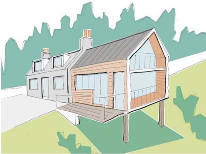
Upgrading and extension to existing whin stone cottage near Gattonside, Scottish Borders. The ground slopes down to the Blake Burn and the new oak frame extension with larch weather boarding and triple glazed windows, deck and upper balcony are supported on oak stilts.
