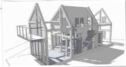
designed to step down with the site levels and to add some extra height in the roof space, which could be used for storage or a deck for sleeping.
